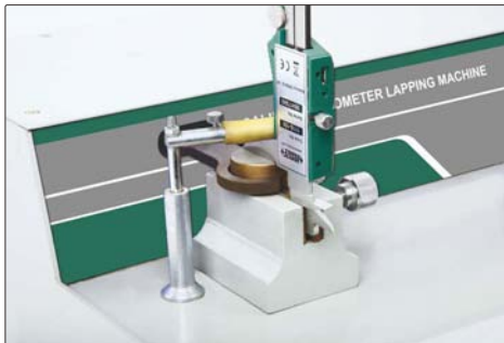
lapping measuring surfaces of caliper lower jaws
