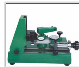
inspect accuracy of test indicators
