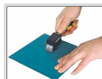
step 1: make grid cutting on surface
