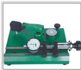
inspect accuracy of dial indicators (range 0-25mm)
