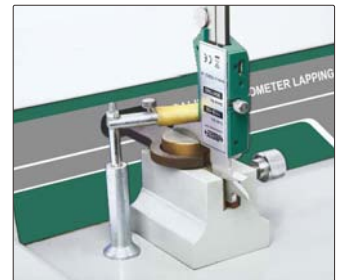
lapping measuring surfaces of caliper lower jaws
