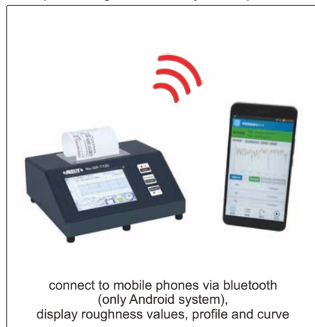
operate roughness tester by mobile phones
