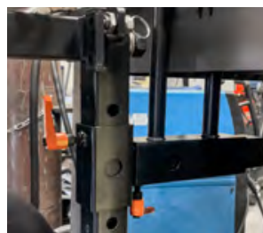
Height adjustment: 2" Extends: 3"
