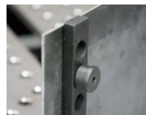
Magnet keeps sheet metal in vertical position
